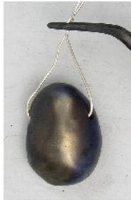
This rock was held by the wire and heated gradually with a torch until it turned dark blue. After quenching it looked like hematite.
