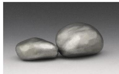
Because of most steel clays' high shrinkage rate, when fired on their own (not in combination with other metals), inside carbon, cracks and distortions may occur. This is caused mainly because of friction with the carbon. The more complex the piece is, the more chance that distortion will happen. This is especially the case with rings. To avoid this, you can fire inside a cage.
