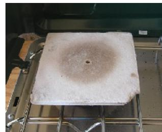
Turn the flame on to full capacity. It will take 3-5 minutes for carbon to heat up. After a few minutes you will smell and see the smoke coming out of the holes in the lids. This is the binder burning. It is important that the binder burns slowly, without catching fire, or pieces will crack. If pieces catch fire, lower the flame. If you are not sure there is smoke, you can lift the lid with a glove or tweezers and look inside.
